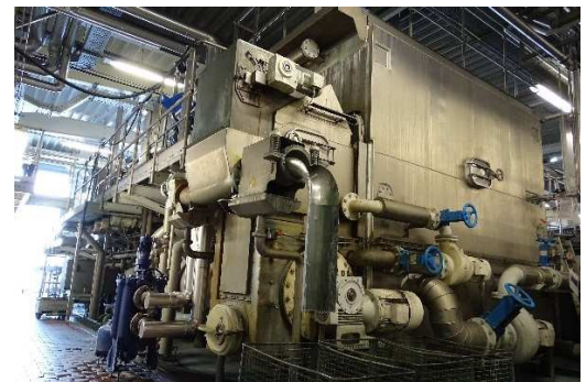
KRONES bottle washing machine Type Lavatec KES 3-4, 46,000 bottles/h
