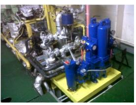
Starboard Bollfilter main engine fuel filter type 6.72.1
