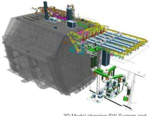
3D Model showing SW System and Shell and Tube Type Vaporizers
