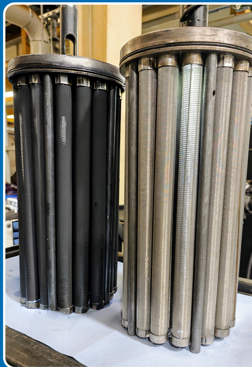
Fouled Candle elements (left) alongside professionally cleaned elements
