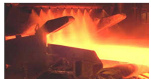
Descal Spray Header
