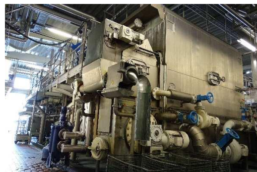
Fig. 2: KRONES bottle washing machine Type Lavatec KES 3-4, 46,000 bottles/h
