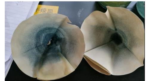
TSS test by ABInBev lab before and after starting using the BOLLFILTER?
