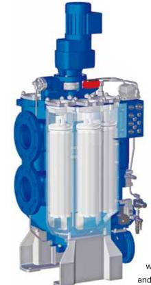
takes over the task of the isolated chamber. The individual filter chambers are subjected to the filtering and backflushing process one after the other in sequence. As a result, filters never reach critical contamination levels.
