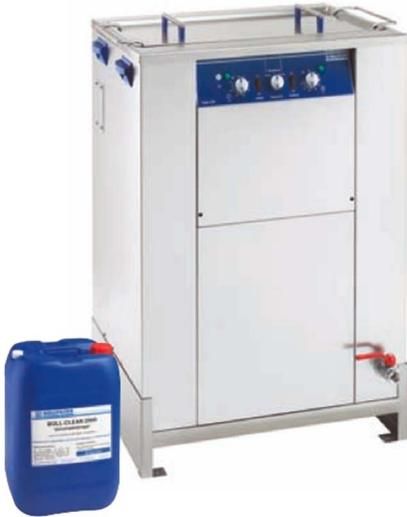
Fine cleaning method for contaminated filter elements with sieve meshes. Highly energetic liquid jets remove virtually all ingrained dirt particles from the mesh of the filter screen. Ultrasonic cleaning is the simple, clean and effective method to restore filter meshes to their original filtration level, open condition.
