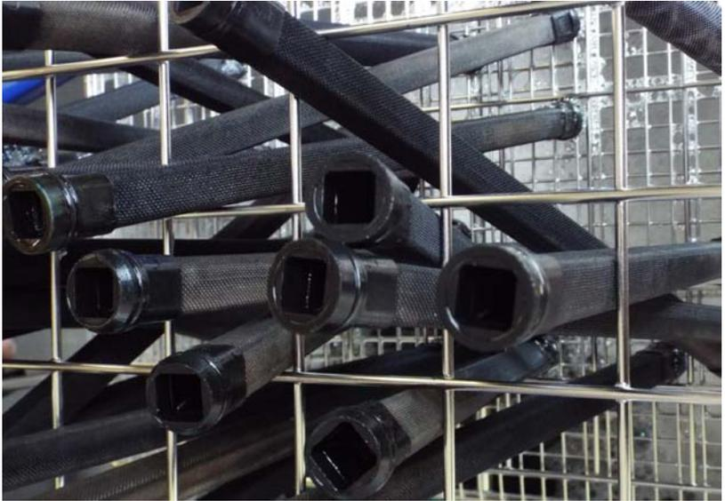
Candles from BOLL 6.46 Lube Oil Filter encrusted with Oil sludge before cleaning
